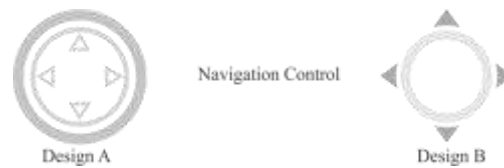
Fig. 12. A noisy navigation control (A) is converted to a minimalist control (B)
